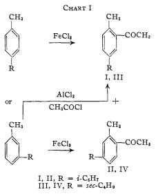
*m*-Cymene was acetylated with ferric chloride as the catalyst to yield II. This ketone formed a (6) H. Pines and A. W. Shaw, J. Org. Chem., **20**, 373 (1955).
